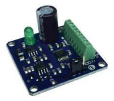
The MBDC050-024031 driver is designed to drive DC brush motors at peak currents of up to 3.0A and 35V. An optional external potentiometer (10K) or external voltage (0.5-5VDC) can be used to control the speed as well. The direction of the motor can be present by the direction control input. To disable energy from the motor, there is a Freewheel input that can be grounded.
